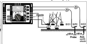
Selective measurement at high voltage pylons:
