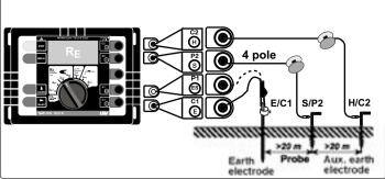
Earth resistance measurement at high voltage pylons:
